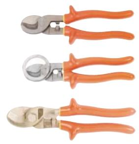
High leverage cutters with shear type blades for cutting 100 pair telephone cable, 4/0 aluminum, and 2/0 copper. Cutter with ring meets Bell spec number R3371D2.
