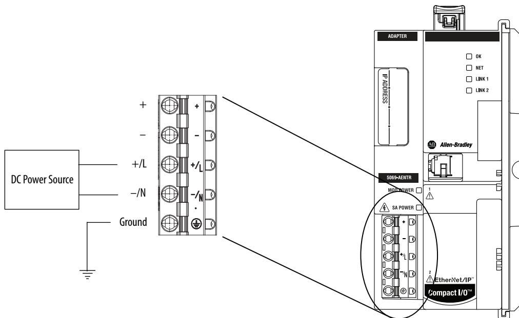
This figure shows a wiring diagram for how to connect SA power (AC) to the 5069-AENTR EtherNet/IP adapter.
