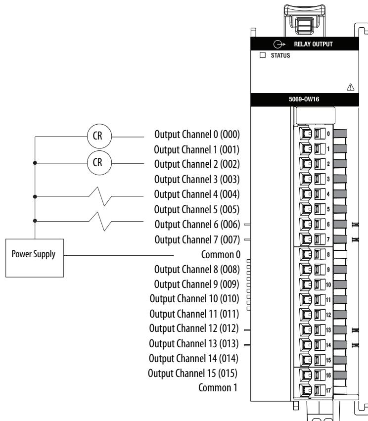
This figure shows a functional block diagram for the 5069-OW16 module.
