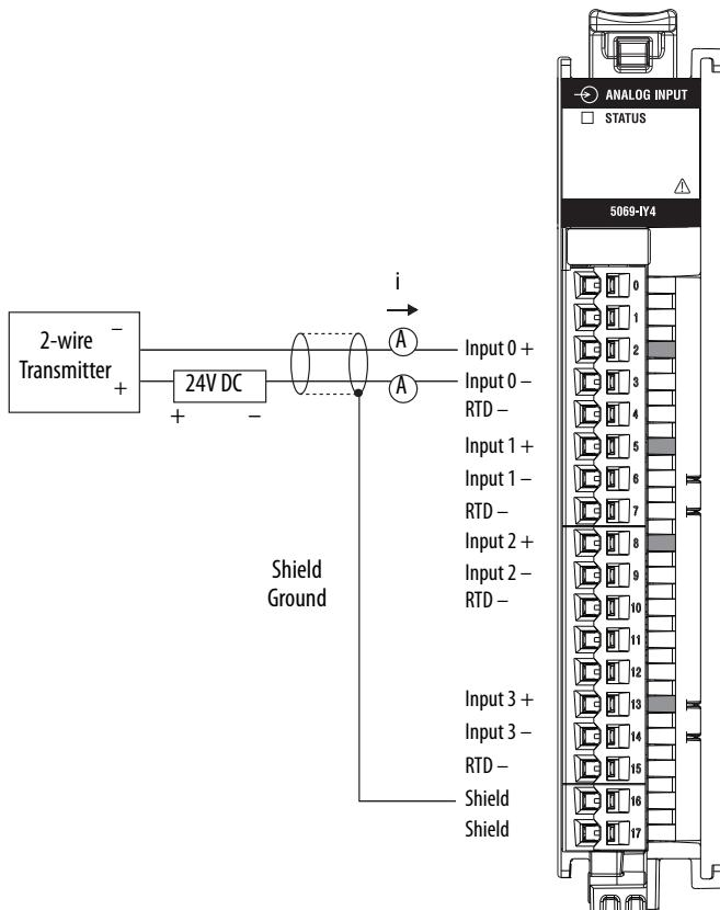
This figure shows a wiring diagram for the 5069-IY4 module when used in voltage mode.
