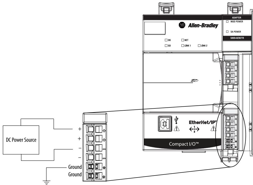
This figure shows a wiring diagram for how to connect SA power (AC) to the 5069-AEN2TR EtherNet/IP adapter.
