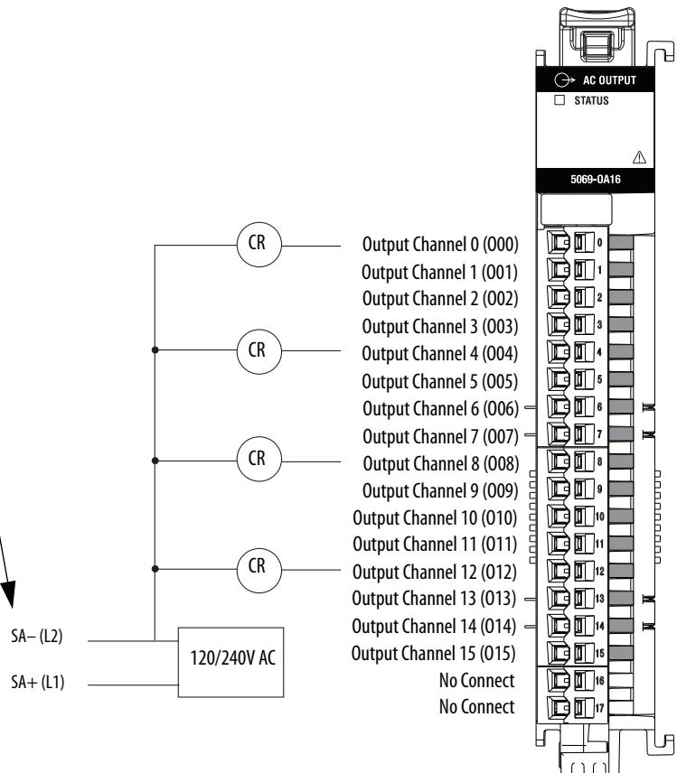
This figure shows a functional block diagram for the 5069-OA16 module.
