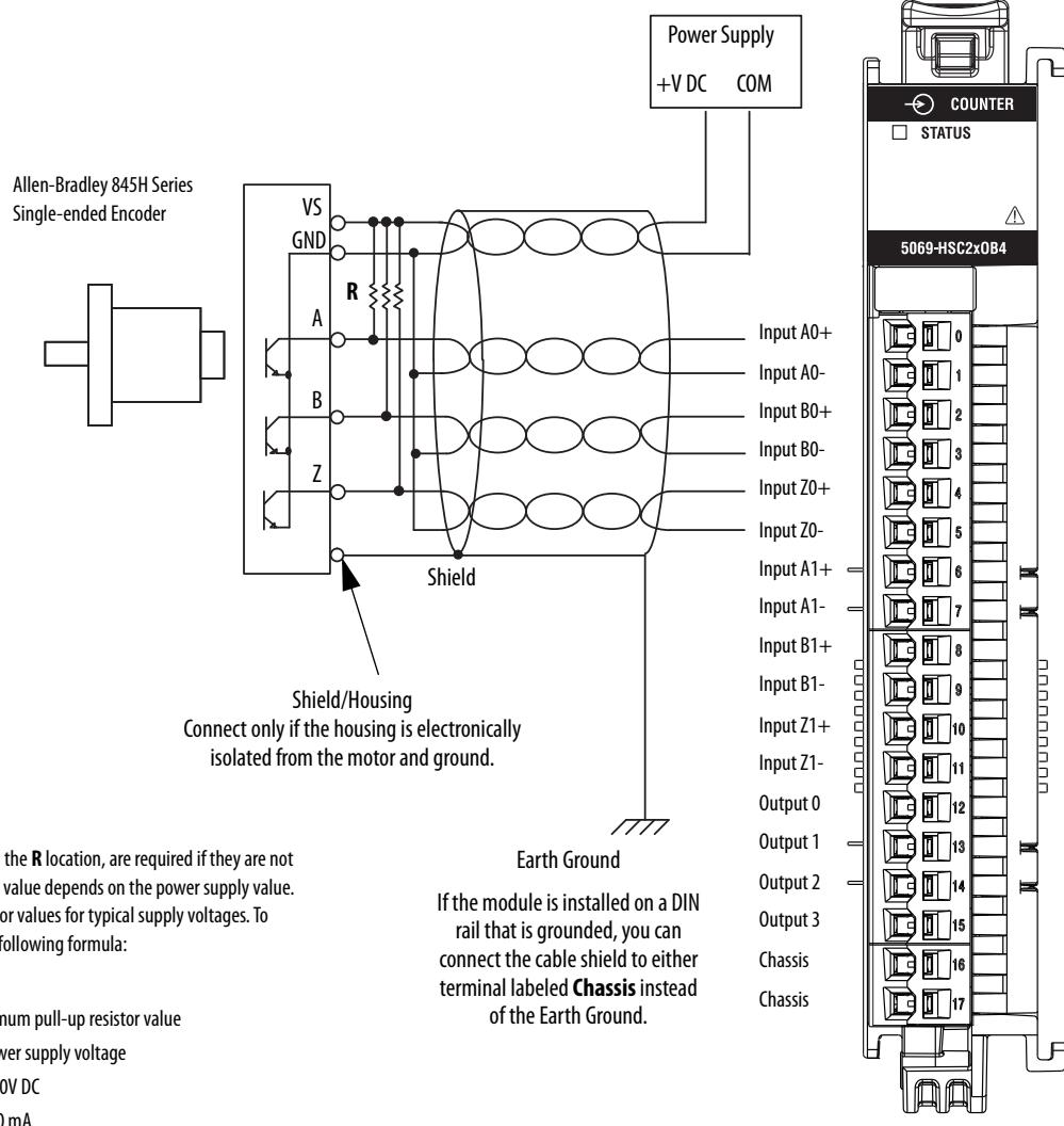
**IMPORTANT:** External resistors, as indicated in the R location, are required if they are not internal to the encoder. The pull-up resistor (R) value depends on the power supply value. The following table shows the maximum resistor values for typical supply voltages. To calculate the maximum resistor value, use the following formula:
