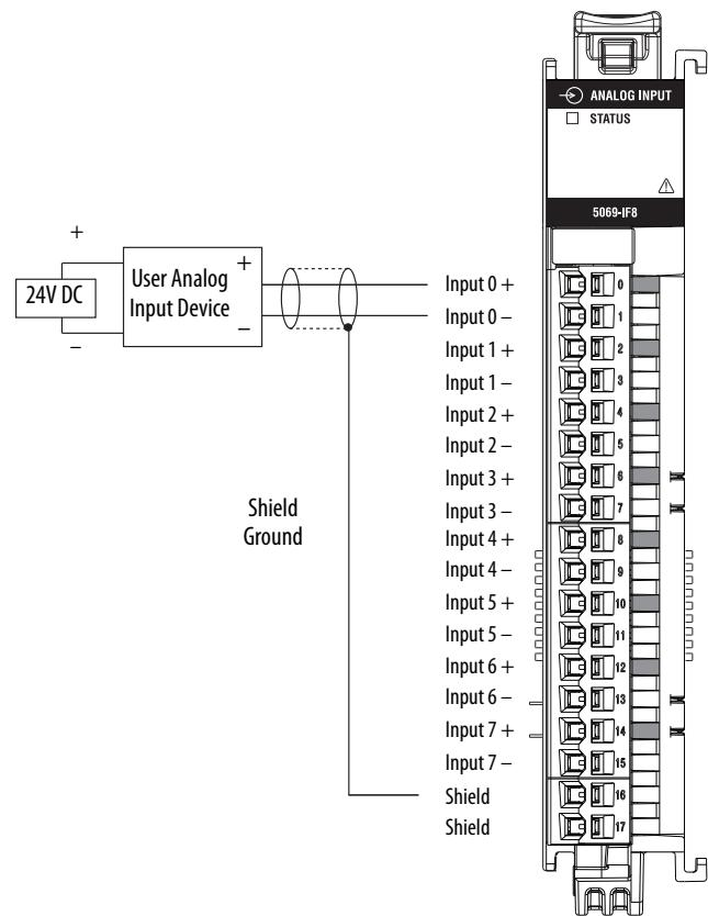
This figure shows a functional block diagram for the 5069-IF8 module.
