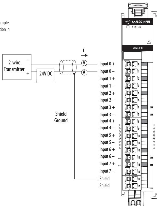
This figure shows a wiring diagram for the 5069-IF8 module when used in voltage mode.
