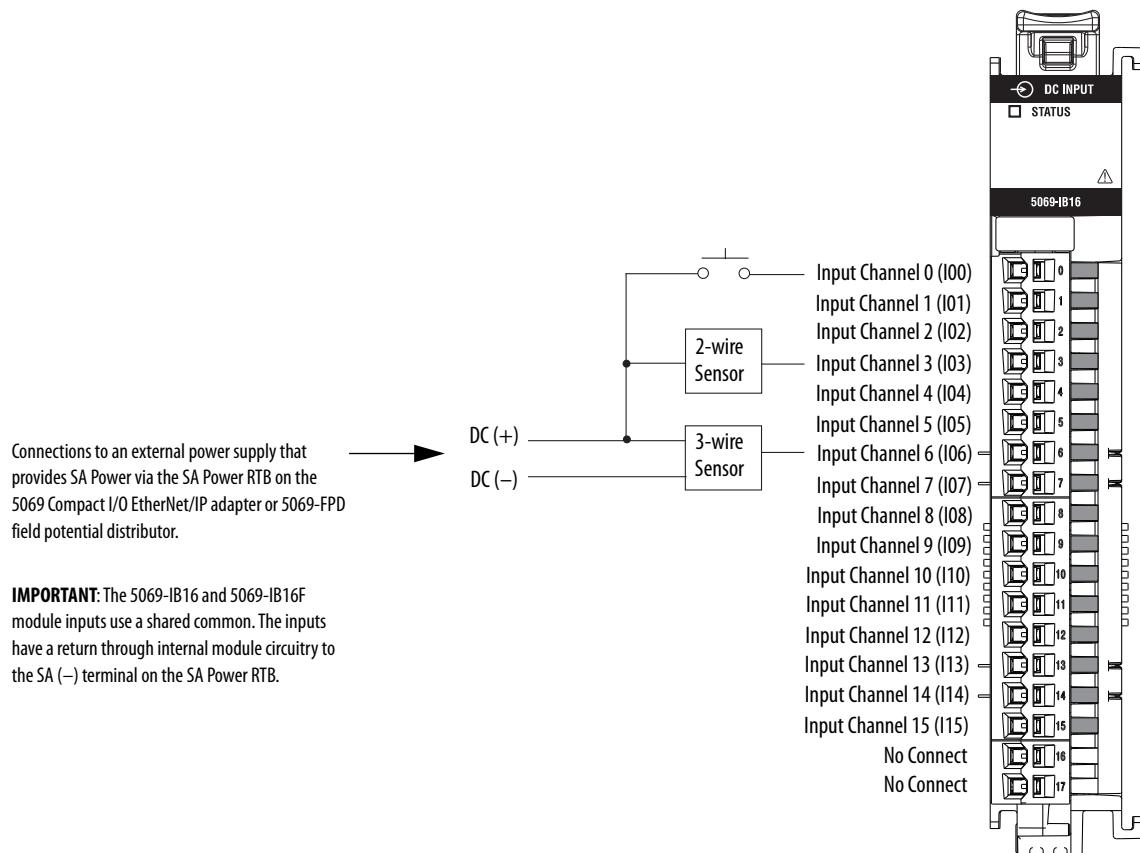
This figure shows a functional block diagram for the 5069-IB16 and 5069-IB16F modules.
