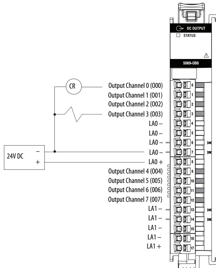
This figure shows a functional block diagram for the 5069-OB8 module.
