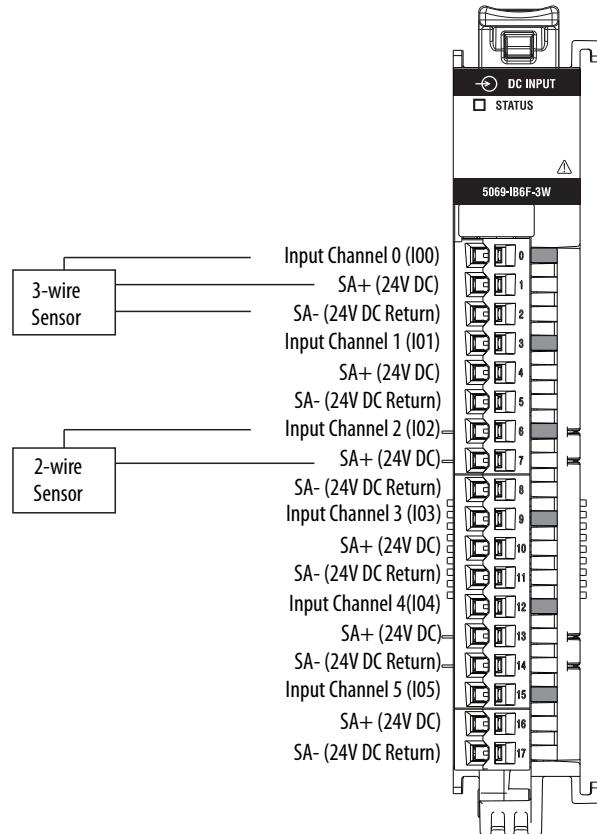
This figure shows a functional block diagram for the 5069-IB6F-3W module.
