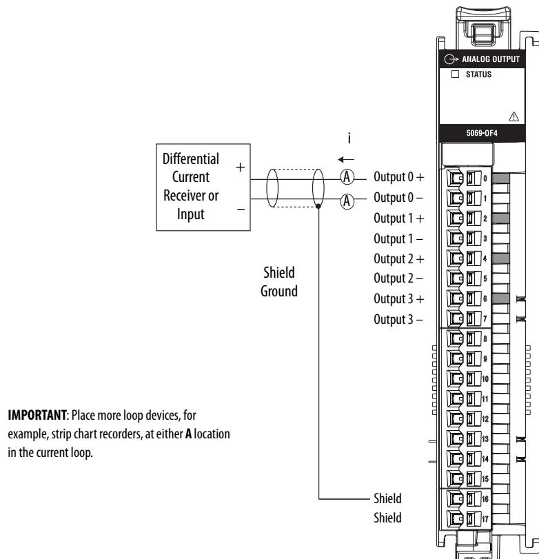
This figure shows a wiring diagram for the 5069-OF8 module when used in current mode.
