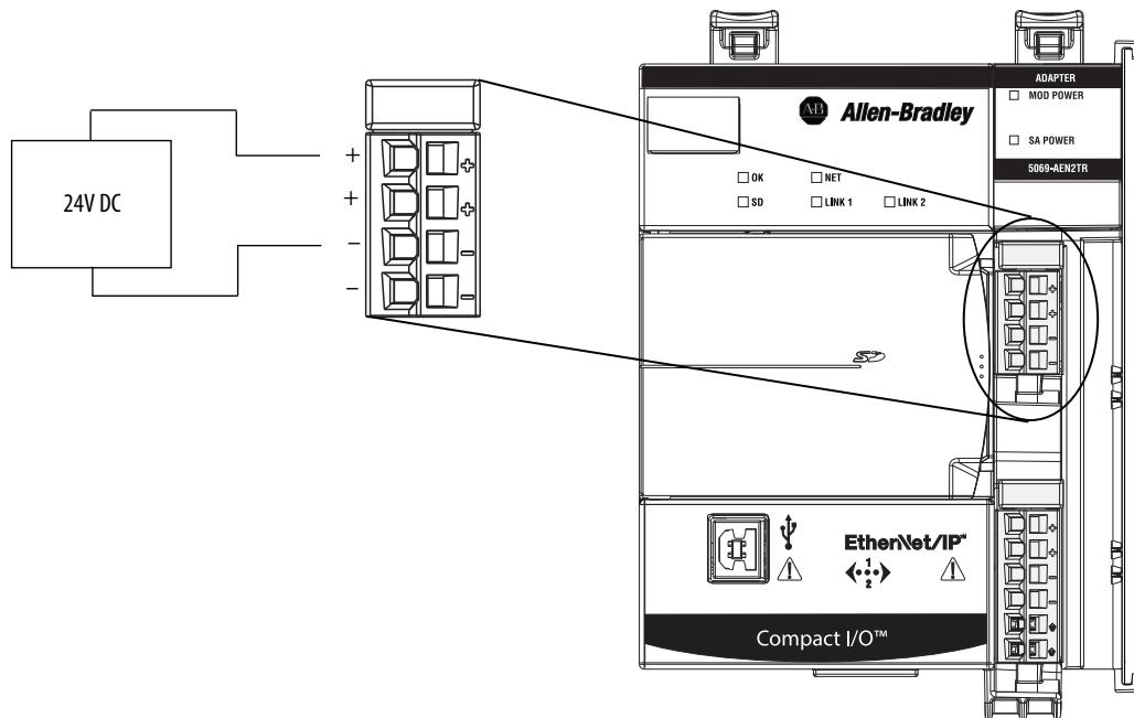
This figure shows a wiring diagram for how to connect SA power (DC) to the 5069-AEN2TR EtherNet/IP adapter.
