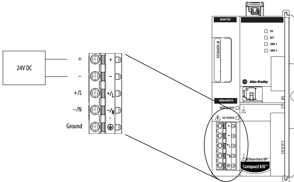
This figure shows a wiring diagram for how to connect SA power (DC) to the 5069-AENTR EtherNet/IP adapter.
