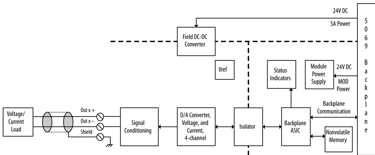
This figure shows a functional block diagram for the 5069-OF8 module.
