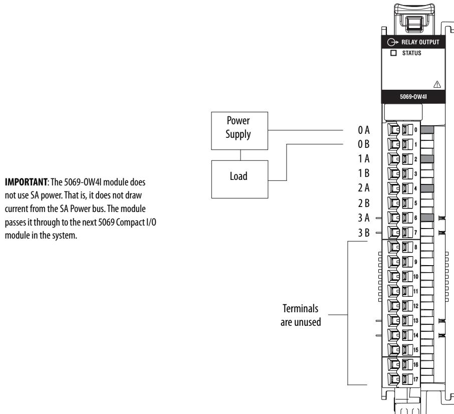
This figure shows a functional block diagram for the 5069-OW4I module.
