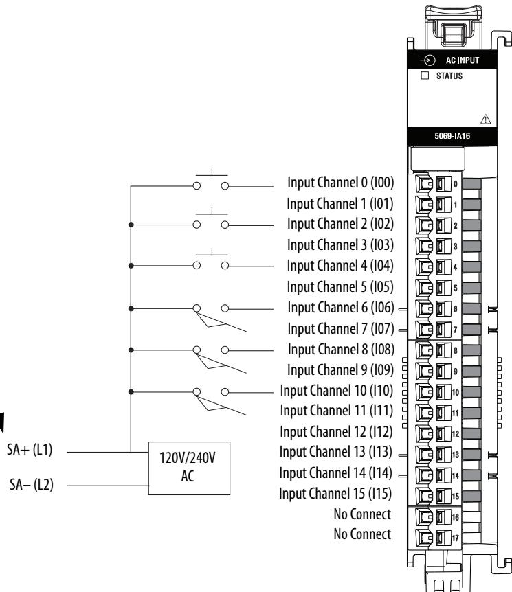
This figure shows a functional block diagram for the 5069-IA16 module.
