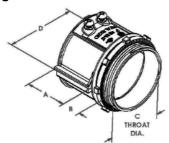
Dimension A in Inches: 2.36 Dimension B in Inches: 1.07 Dimension C in Inches: 4.02 Dimension D in Inches: 4.37
