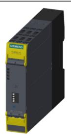
SIRIUS SAFETY RELAY BASIC UNIT ADVANCED SERIES WITH TIME DELAY 0.5-30S ELECTRONIC ENABLING CIRCUITS 2 INSTANTANEOUS 2 DELAYED US = 24 V DC SPRING-LOADED TERMINAL
