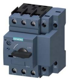
CIRCUIT-BREAKER SZ S0, FOR MOTOR PROTECTION, CLASS 10, W. OVERLOAD RELAY FUNCTION A-RELEASE 27...32A, N-RELEASE 400A, SCREW CONNECTION, STANDARD SW. CAPACITY
