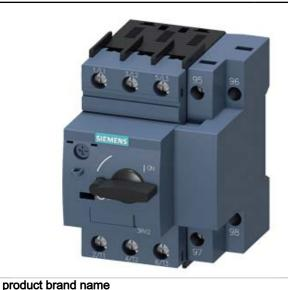
CIRCUIT-BREAKER SZ S00, FOR MOTOR PROTECTION, CLASS 10, W. OVERLOAD RELAY FUNCTION A-RELEASE 1.1...1.6A, N-RELEASE21A, SCREW CONNECTION, STANDARD SW. CAPACITY
