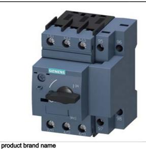
CIRCUIT-BREAKER SZ S00, FOR MOTOR PROTECTION, CLASS 10, W. OVERLOAD RELAY FUNCTION A-RELEASE 0.18...0.25A, N-RELEASE3.3A SCREW CONNECTION, STANDARD SW. CAPACITY
