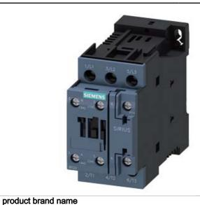
COUPLING RELAY, AC-3, 11KW/400V, 1NO+1NC, DC 24V, W. PLUGGED-IN VARISTOR 3-POLE, SZ S0 SCREW TERMINAL
