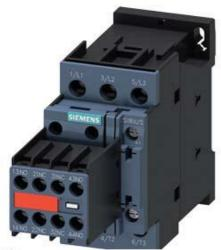
CONTACTOR, AC-3, 7.5KW/400V, 2NO+2NC AC110V 50HZ/120V 60HZ 3-POLE, SZ S0 SCREW TERMINAL PERMANENT AUX. SWITCH FOR SUVA APPLICATIONS
