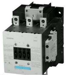
CONTACTOR, 275A/AC-1, AC(40...60HZ)/DC OPERATION UC 220...240V AUXIL. CONTACTS 2NO+2NC 3-POLE, SIZE S6 BAR CONNECTIONS CONVENT. OPERATING MECHANISM
