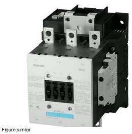
CONTACTOR, 90KW/400V/AC-3, AC(40...60HZ)/DC OPERATION UC 21...27.3V AUXIL. CONTACTS 2NO+2NC 3-POLE, SIZE S6 BAR CONNECTIONS ELECTRONIC OPERATING MECHANISM WITH 24V DC PLC INTERFACE SCREW TERMINAL
