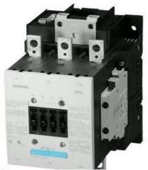
CONTACTOR, 55KW/400V/AC-3 AC(40...60HZ)/DC OPERATION UC 21...27.3V AUXIL. CONTACTS 2NO+2NC 3-POLE, SIZE S6 BAR CONNECTIONS ELECTRONIC OPERATING MECHANISM WITH PLC INTERFACE 24V DC SCREW TERMINAL
