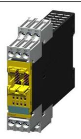
SIRIUS, EXPANSION MODULE 3RK32 FOR MODULAR SAFETY SYSTEM 3RK3 2/4 F-DI, 2 F-DO, 24V DC/1.2A PARAMETERIZABLE VIA SW MSS ES WIDTH 22.5MM SCREW TERMINAL UP TO SIL3 (IEC 61508) UP TO PERFORMANCE LEVEL E (ISO 13849-1)
