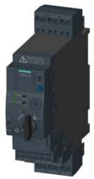
SIRIUS, COMPACT STARTER, DIRECT STARTER 690 V, 24 V AC/DC, 50 ... 60 HZ, 0.1 ... 0.4 A, IP20, CONNECTION MAIN CIRCUIT: SPRING-LOADED TERMINAL, CONNECTION AUXILIARY CIRCUIT: SPRING-LOADED TERMINAL
