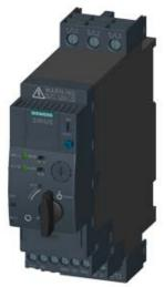
SIRIUS, COMPACT STARTER, DIRECT STARTER 400 V, 110 ... 240 V AC/DC, 50 ... 60 HZ, 8 ... 32 A, IP20, CONNECTION MAIN CIRCUIT: SCREW TERMINAL, CONNECTION AUXILIARY CIRCUIT: SCREW TERMINAL
