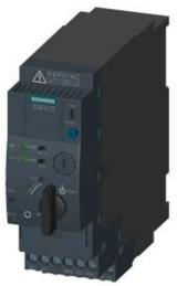
SIRIUS, COMPACT STARTER, DIRECT STARTER 690 V, 110 ... 240 V AC/DC, 50 ... 60 HZ, 1 ... 4 A, IP20, CONNECTION MAIN CIRCUIT: PLUGGABLE, WITHOUT TERMINALS, CONNECTION AUXILIARY CIRCUIT: SCREW TERMINAL
