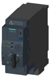
SIRIUS, COMPACT STARTER, DIRECT STARTER 400 V, 110 ... 240 V AC/DC, 50 ... 60 HZ, 8 ... 32 A, IP20, CONNECTION MAIN CIRCUIT: PLUGGABLE, WITHOUT TERMINALS, CONNECTION AUXILIARY CIRCUIT: PLUGGABLE, WITHOUT TERMINALS
