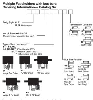
\*Angle Bar mounts on common or center terminals only. \*\*SL Version is not available with bus bars. †Minimum of 4 Poles Required. \*\*\*.38 max. leads if not specified.
