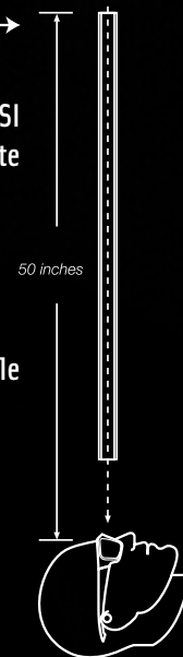
Diagram of High Mass Impact and Penetration Tests
