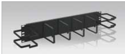
Metal Ring Panel ICCMSCMP32 3.5" H x 19" W, 1 rack mount space • 4 vertical and 4 horizontal rings • Includes #12 rack screws
