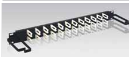
Metal Ring Panel with Routing Clips ICCMSCMP41 1.75" H x 19" W, 1 rack mount space • 2 vertical rings with 24 routing clips • Includes #12 rack screws
