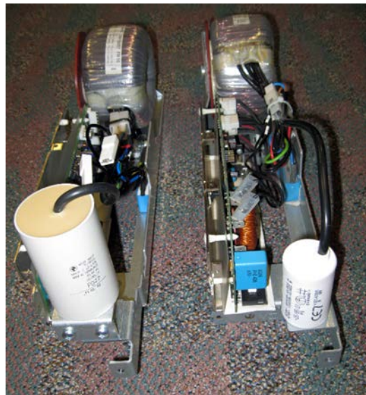
Series B Capacitor in a Right-side AC Fan Inverter Assembly Shown.
