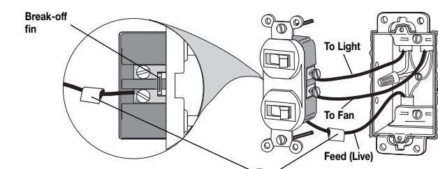
MARK or TAG the wire that is connected to the feed side of the switch (the side with the break-off fin).
