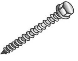
An externally threaded, hardened screw with a double lead, consisting of alternating raised and lowered threads with notches cut into the raised threads, and a diamond-shaped, nail-type point.
