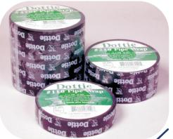
Soft PVC pipe wrap/corrosion prevention tapes are coated on SPVC films with an aggressive rubber-based pressure sensitive adhesive, in 10 mil (x10) and 20 mil (x20) thickness, black color and matte finish, compliant to IAPMO-UPC in either blank or printed with UPC logo.
