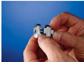
1. Loosen nut and open clamp.
