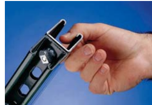
2. Position strut back-to-back and push STS clamp into slot. Rotate 90 degrees.
