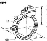
**Download Photo Image** Dimension A in Inches: 4.18 Dimension B in Inches: 5.61 Dimension C in Inches: 1.13 Dimension D in Inches: 7.15 O.D. Dimension E in Inches: 5.85 I.D.
