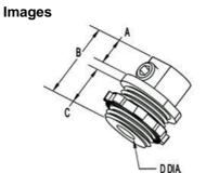
Download Photo Image Dow Dimension A in Inches: .56 Dimension B in Inches: 1.25 Dimension C in Inches: .56 Dimension D in Inches: .48
