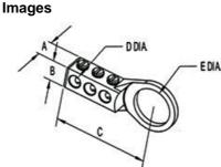
Download Photo Image Dimension A in Inches: .50 Dimension B in Inches: .50 Dimension C in Inches: 1.94 Dimension D in Inches: .26 Dimension E in Inches: .88
