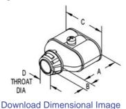
Download Photo Image Dow Dimension A in Inches: 1.63 Dimension B in Inches: .43 Dimension C in Inches: 1.88 Dimension D in Inches: .53
