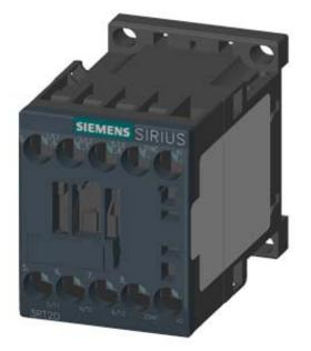
CONTACTOR, AC-3, 3KW/400V, 1NC, AC110V 50HZ, 120V 60HZ 3-POLE, SZ S00 SCREW TERMINAL
